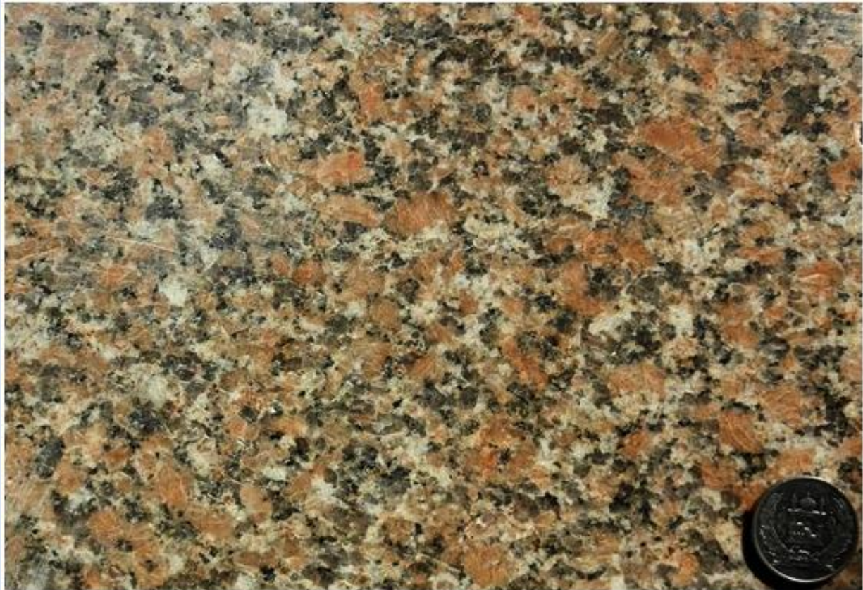
Figure 5 A polished slab of medium grained equigranular granite, comprising >60 vol.% of pinkish orthoclase feldspar.
