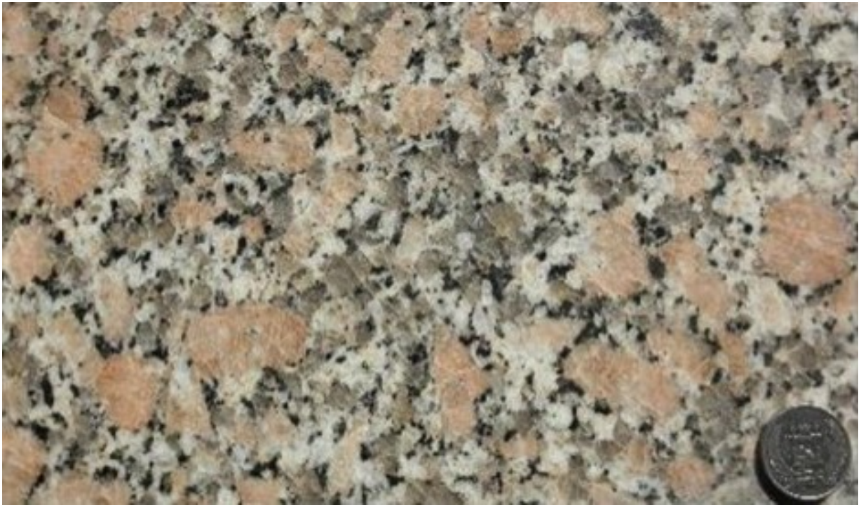
Figure 4. A polished slab of coarse grained porphyritic granite. Abundant coarse grained pinkish orthoclase feldspar embedded in relatively medium-fine grain plagioclase feldspar (grey) and quartz (white) and biotite (dark minerals).
